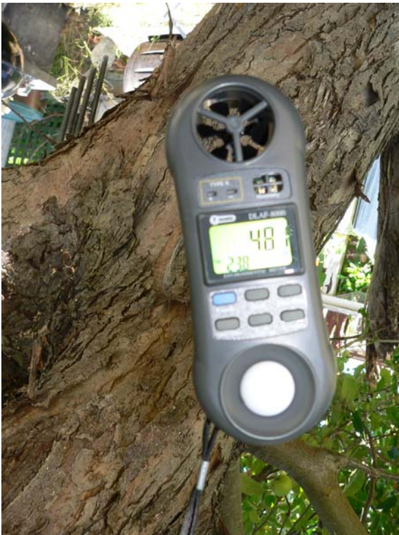
Measuring outdoor relative humidity. It was significantly lower than indoor humidity.
